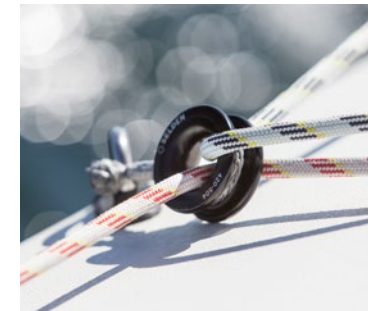
One ring used for gennaker sheet and Code 0 sheet.
