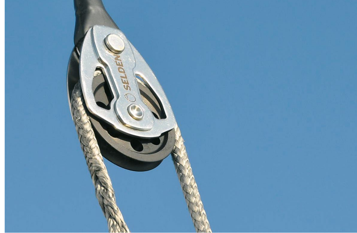
Dyneema core in the bridle is an alternative to 7x19 strand wire.
