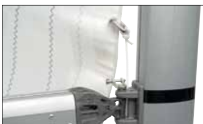
1) Tie the pre-feeder to the boom bracket.
