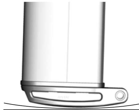
Convex heel plug distributes compression load evenly on the mast section.
