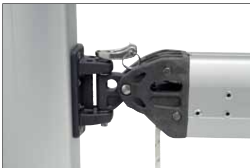
D-shaped head of clevis pin.
