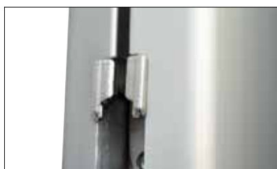
2) Feed the luff rope into the sail entry.
