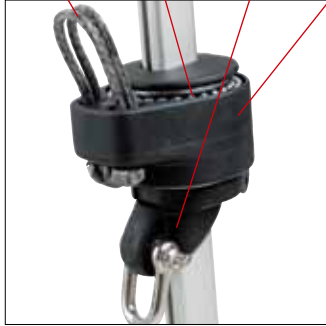
Halyard swivel in composite with stainless steel reinforcement. Low weight (230 g). Low friction due to the load distributor.
