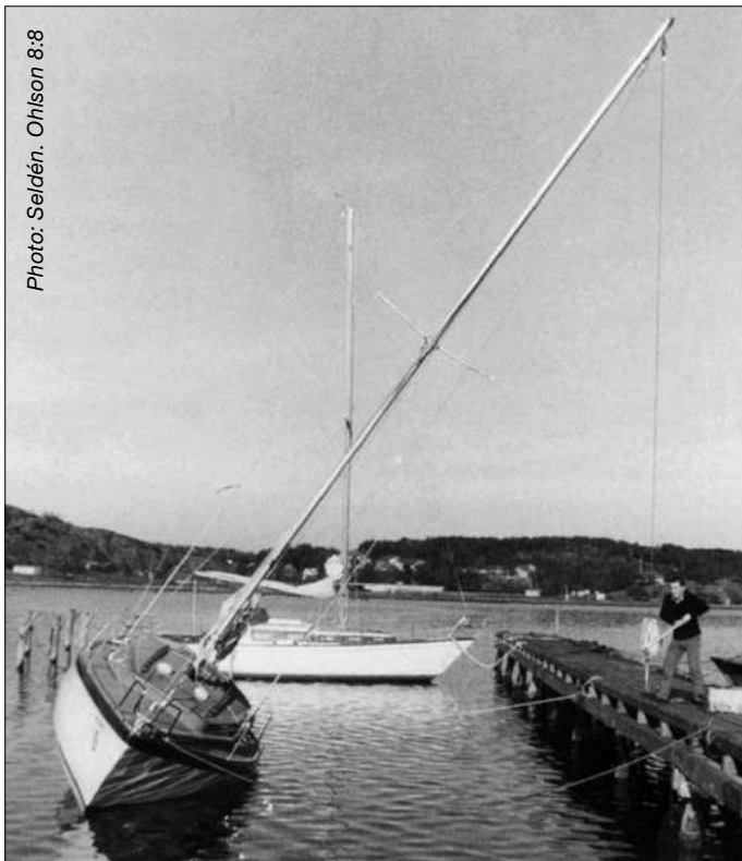
Heeling test in 1971. The righting moment of the boat is measured at 30° heel.
