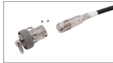
Pull the terminal over the line and fold the core of the line over the wedges. Insert the wedges to the terminal.
